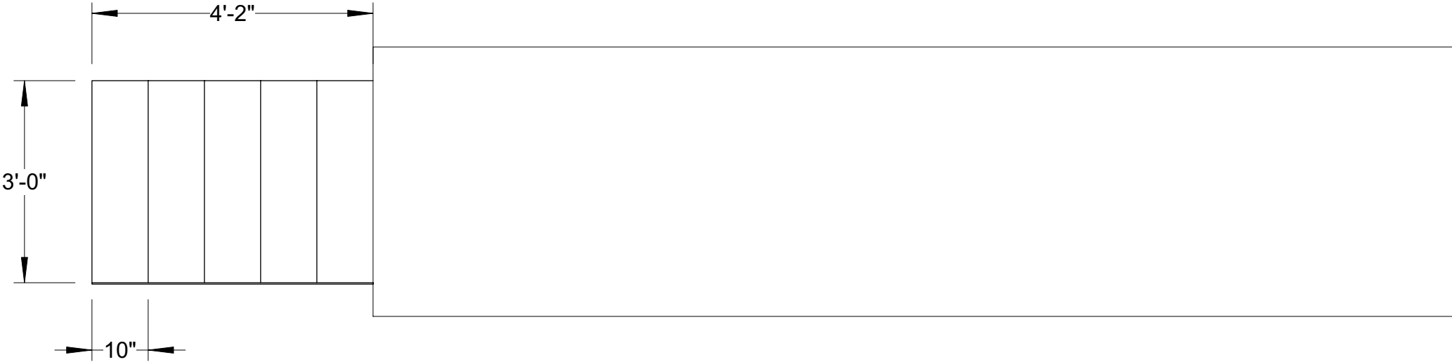
3 BRIDGE PLATFORM CENTER - FRONT VIEW Scale: 1/2"=1'-0"
